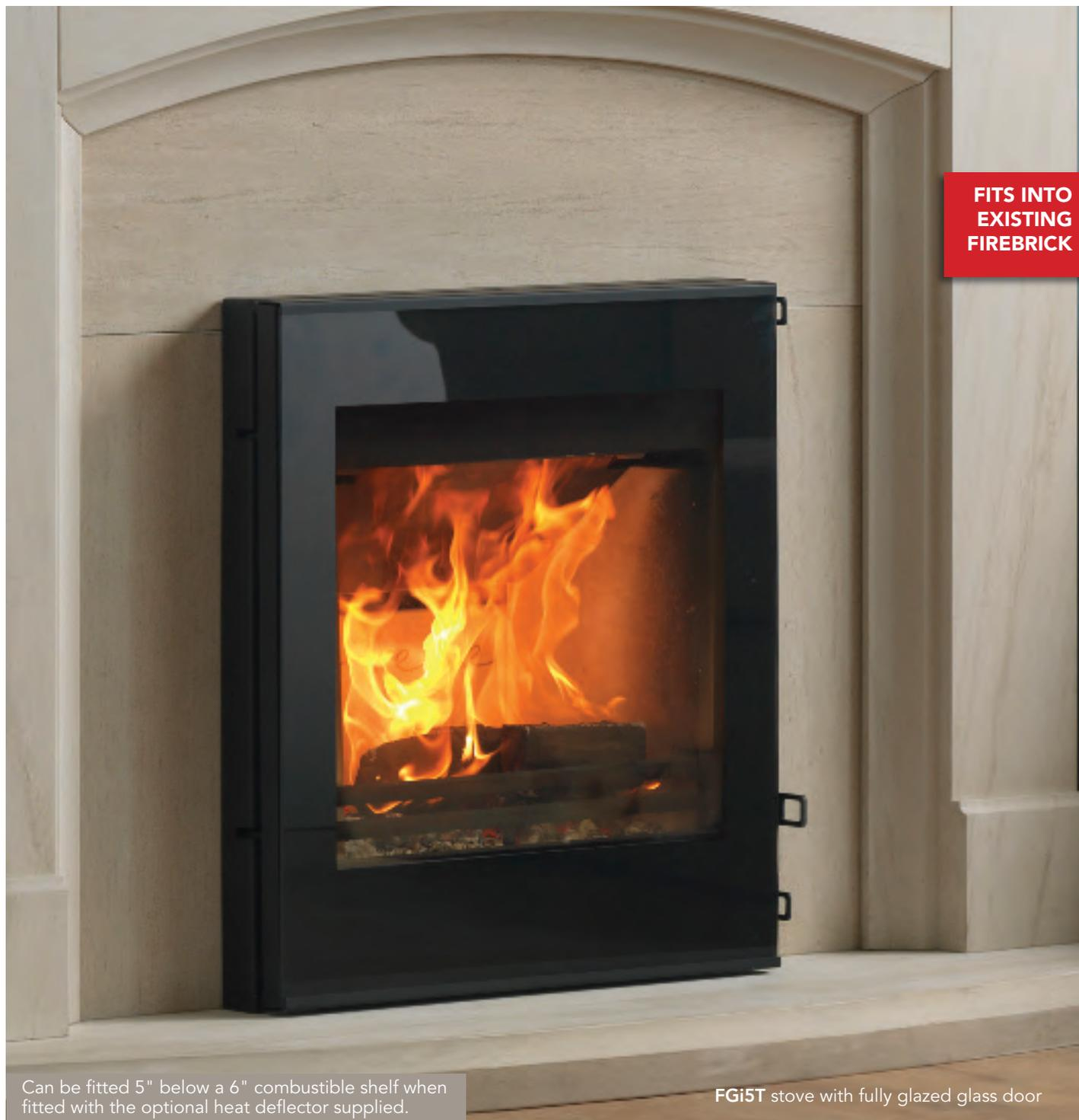
Can be fitted 5" below a 6" combustible shelf when fitted with the optional heat deflector supplied.
